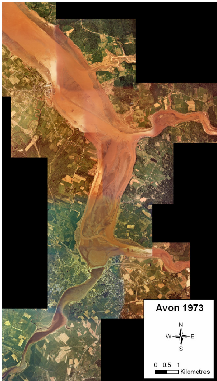
Figure 7: Avon 1973 generated from 1: 16,000 scale aerial photographs. Mosaic ground resolution = 1 m.
