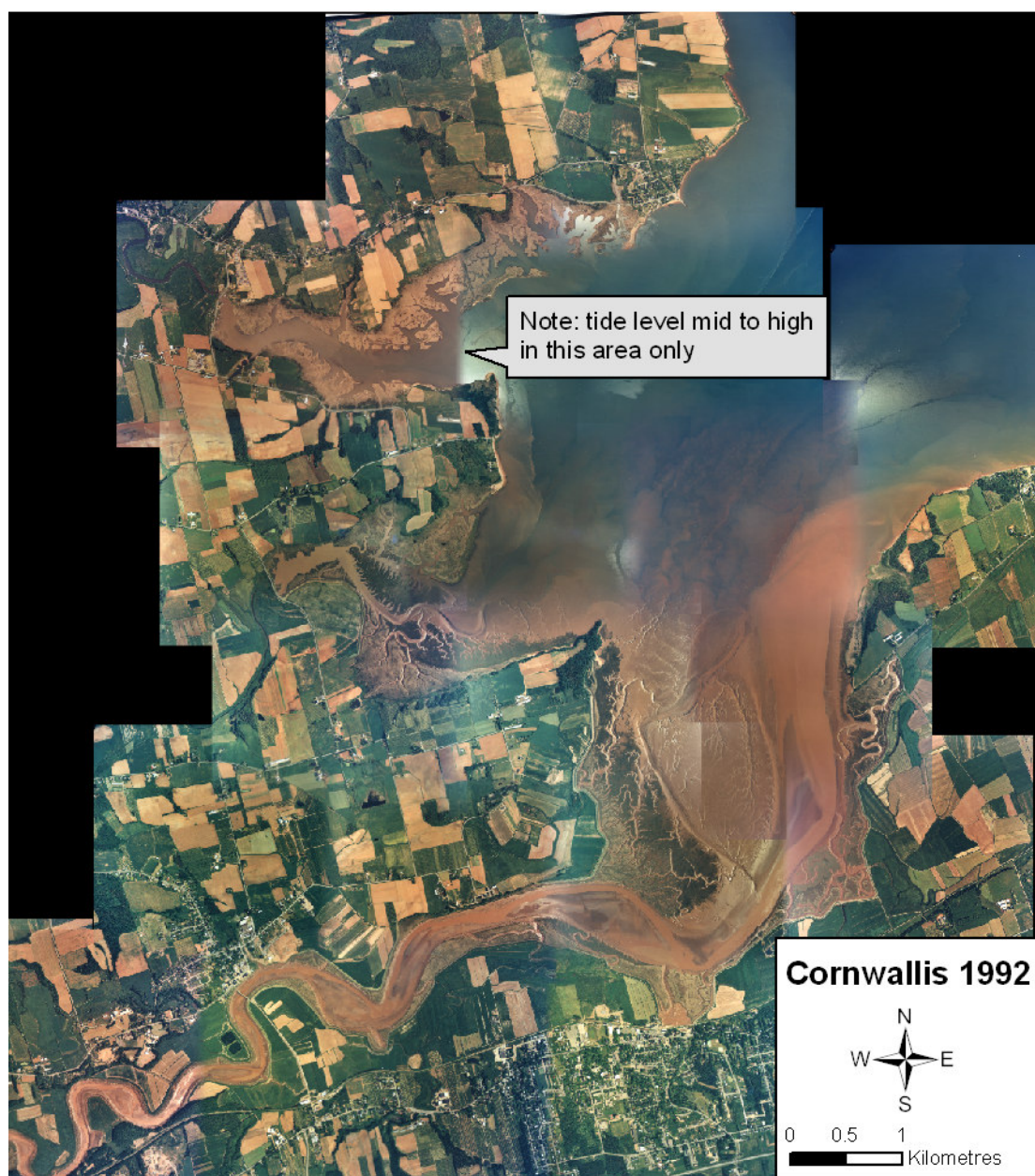
Figure 12: Cornwallis 1992 generated from 1:10,000 scale aerial photographs. Mosaic ground resolution = 1m.
