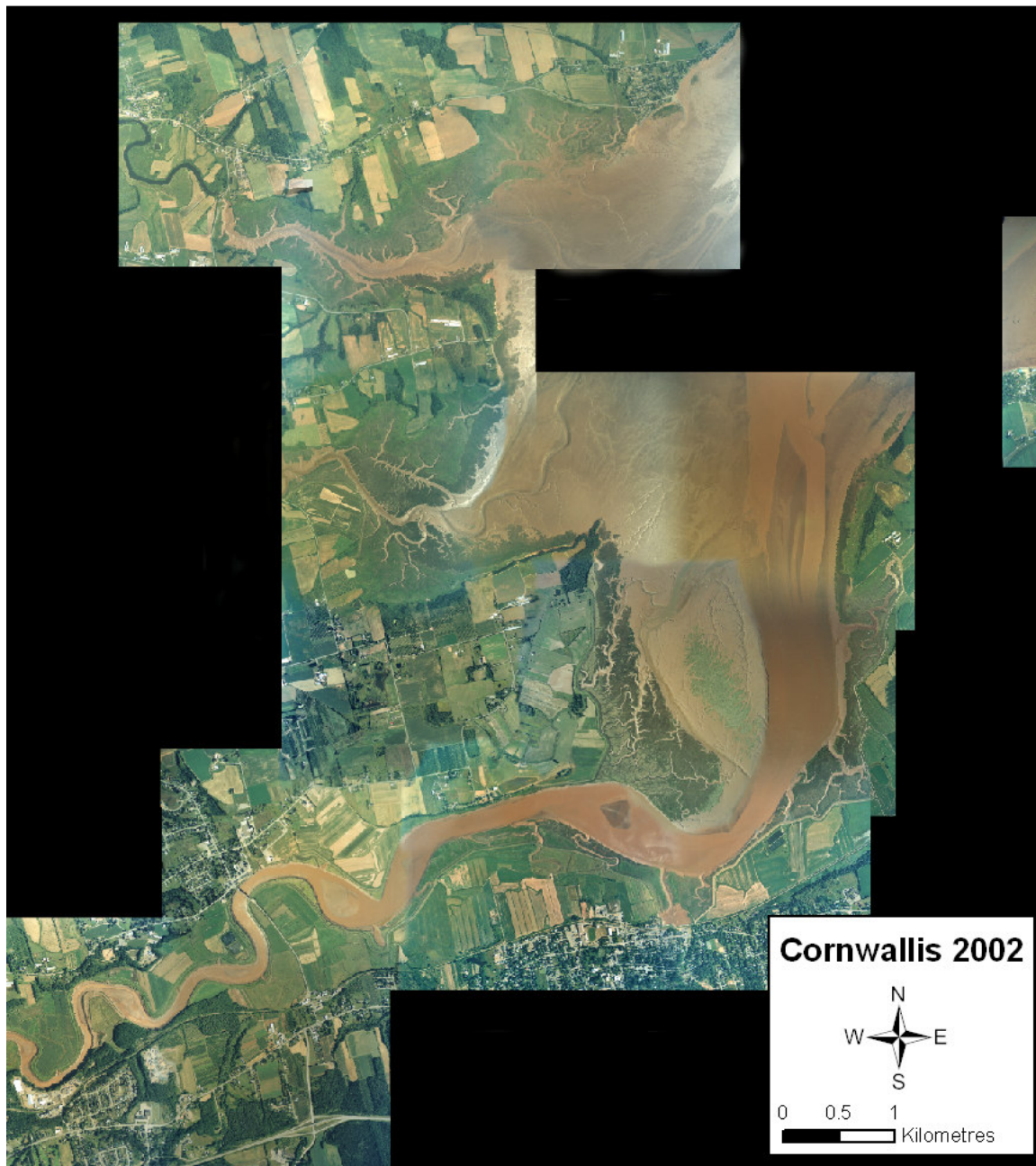
Figure 13: Cornwallis 2002 generated from 1: 10,000 aerial photographs. Mosaic ground resolution = 1m.
