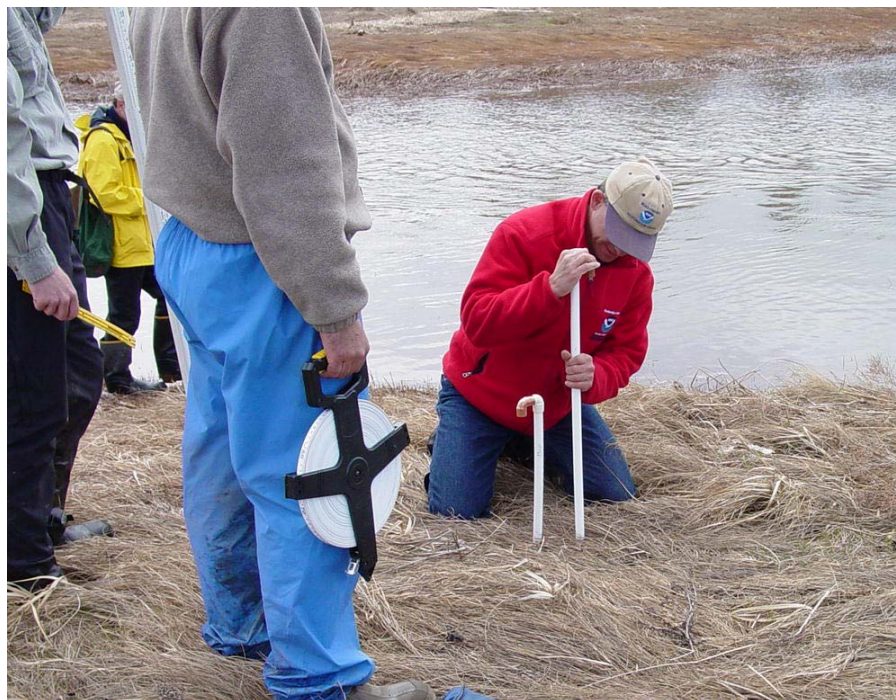
Figure 12 Eric Hutchins (US National Oceanic and Atmospheric Administration: NOAA) demonstrates the proper technique for installing groundwater and salinity wells at Cheverie Creek. Photo by T. Bowron, spring 2003.
