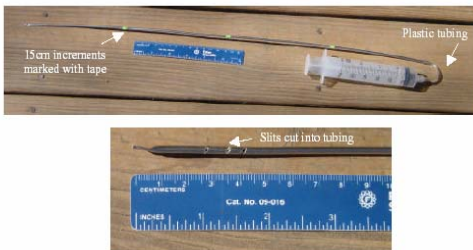
Figure 17 Photograph of a soil probe (sipper) used to sample pore water salinity (Roman et al 2001).
