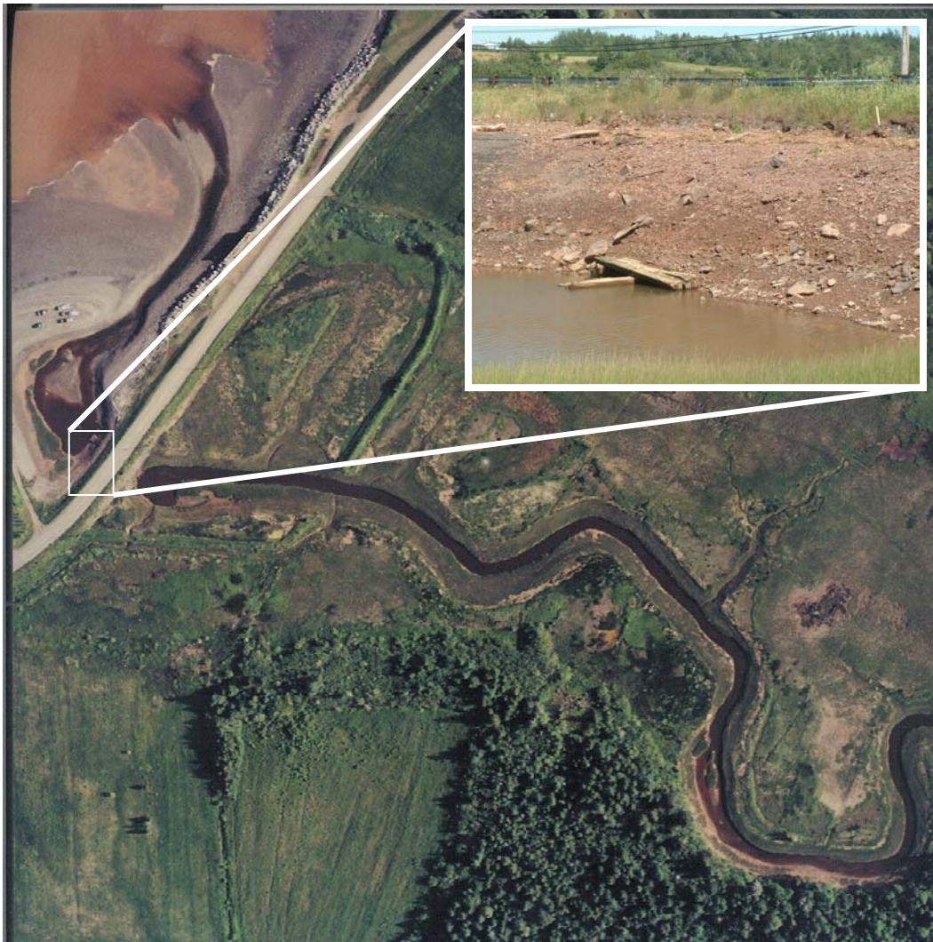
Figure 7 1992 aerial photograph of Cheverie Creek Causeway-Culvert. (Modified from Nova Scotia Department of Natural Resources, 2003). Inserted image is of the two-lane rock-filled causeway and the square wooden box culvert almost completely submerged at low tide by freshwater flow; taken by T. Bowron, 2002.
